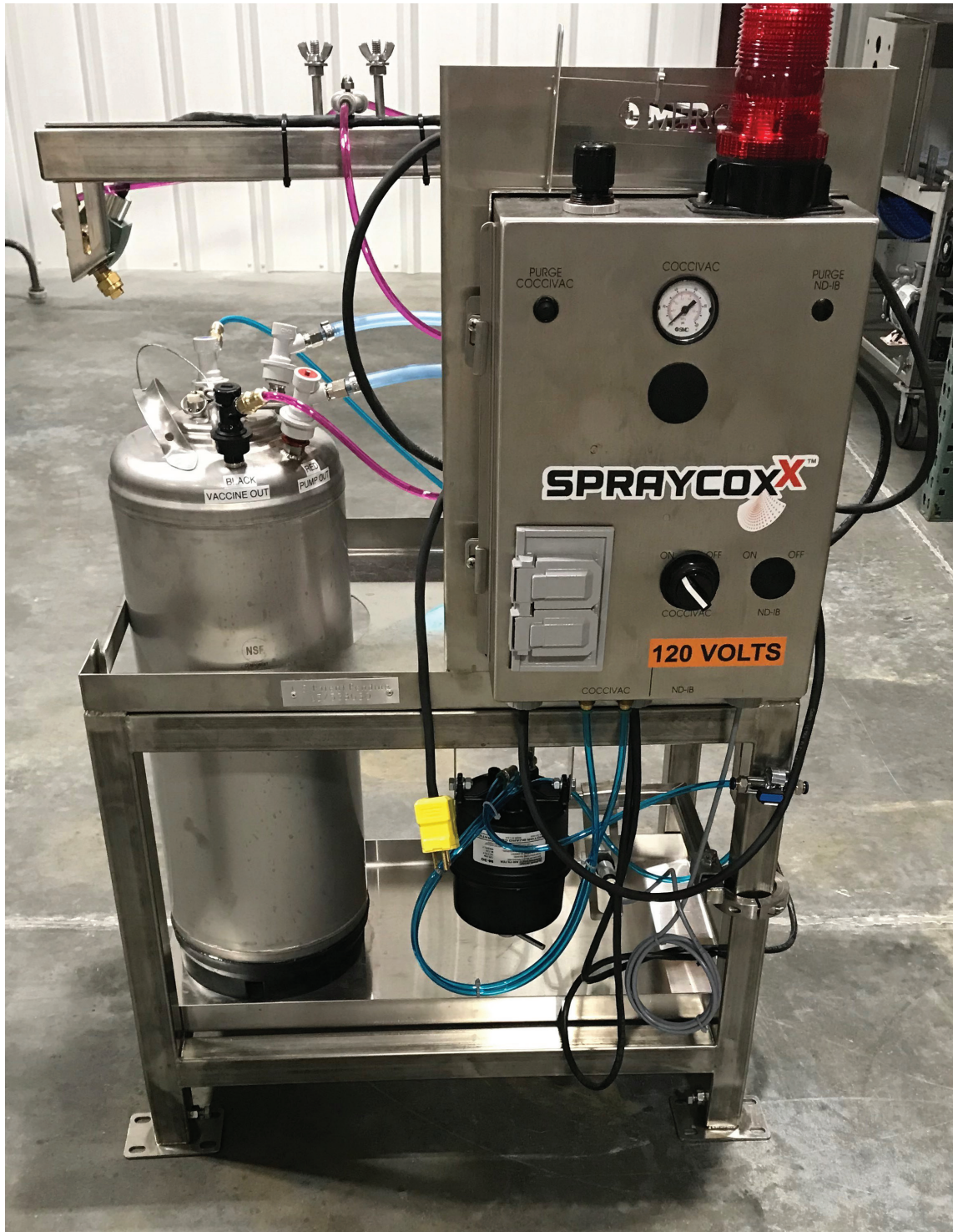
Latest generation Spraycox X spray cabinet for Coccivac application in the hatchery.
