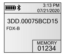
On Unique - A tag ID is stored and transmitted via USB and Bluetooth connections only once when it is detected several times in a row. If another tag is detected after the first tag, and the first tag is detected again, it will be read and stored again. If the reader is powered off and on, the tag ID can be stored and transmitted again. On Unique is the default Memory setting. See examples on the following page.
