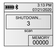
• The reader will automatically power off after a certain period of inactivity. The inactivity time is user adjustable and by default is set to 180 seconds (3 minutes). Pressing any button will reset the timer.
