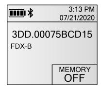
On All - All detected tag IDs will be stored in the memory and transmitted via USB and Bluetooth connections. The memory counter on the main screen will increase after each detection.
