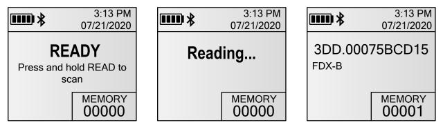
When the READ button is released and no tag has been read, the HPR Lite will generate three short beeps, exit scan mode, and display the message **No tag detected** then return to the last message that was on the main screen.
