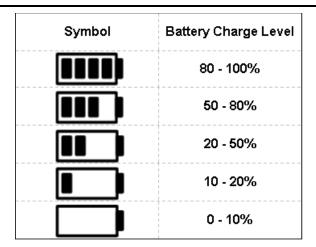
If the reader is powered on while the battery level is at or below 10%, the unit will display the message Battery Low and will sound three quick beeps.
