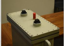
To secure bolts in place, install flat washer between battery box flange and nut for each bolt.
