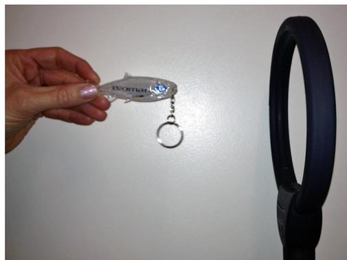
The Antenna and FDX-B Test Tag
