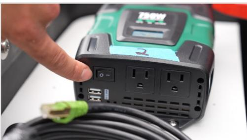
4) On the inverter, turn the power switch to “on.”
