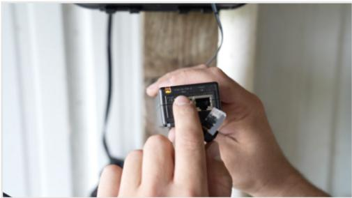
2) Connect the other end of the Ethernet cable to the Power and Data port to the 55v SenseHub power supply that comes in the box with the Controller. Then, connect another Ethernet cable from the “Data Only” port on this power supply to the internet router or network switch. Once connected to the internet, the light on the Controller will turn from red to green.
