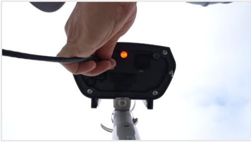
1) Using an Ethernet cable, connect one end of the cable to the PD port on the SenseHub Controller.
