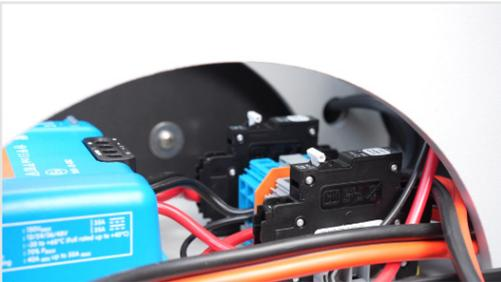
2) Under the inverter, ensure the two breaker switches are switched to the “on” position.
