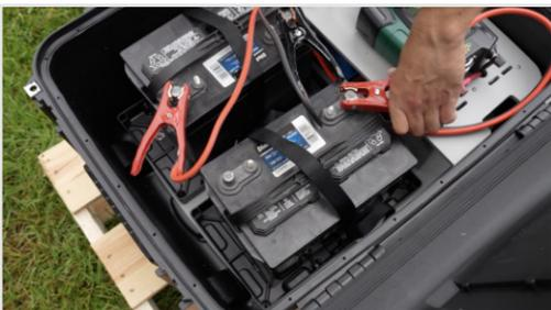
3) Place the two deep cycle batteries inside the case and secure with straps. Attach the power cables to the batteries, ensuring red cables go to the positive terminals and black cables go to the negative terminals.
