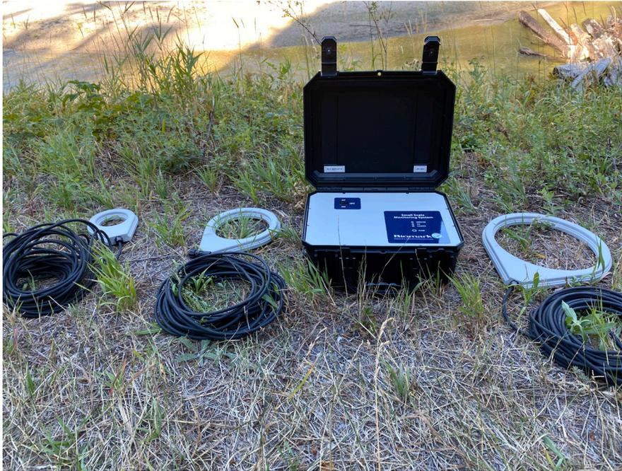
The **SMALL SCALE SYSTEM** is a single reader system that is ideal for terrestrial applications, expands to connect up to 16 antennas, and can be customized for aquatic and submersible applications. Fully custom antenna sizes are also available.
